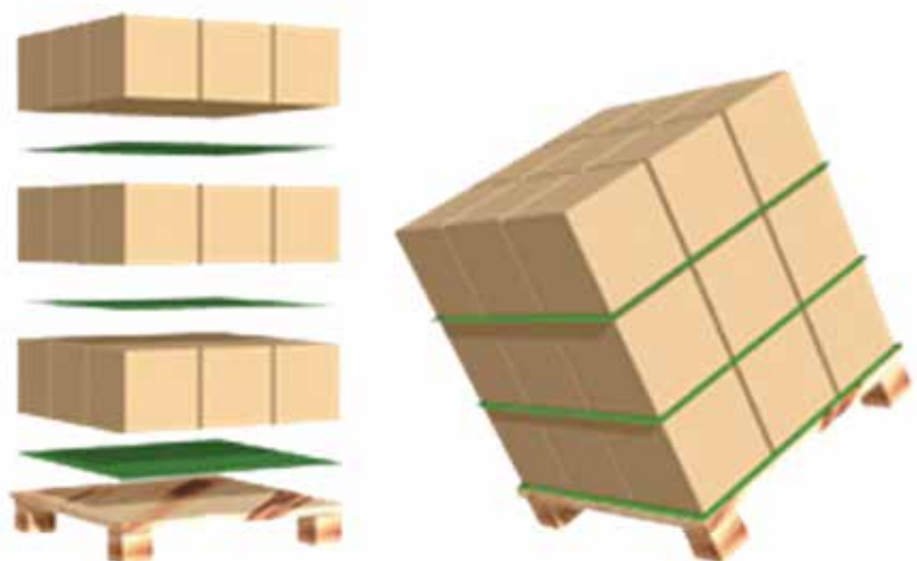
Grip sheets placed in every layer
